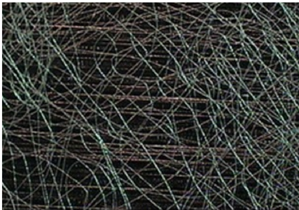
Figure 2: SEM micrographs of silicon wires formed by electrospinning a PMMA/Si 6 H 12 -derived ink
